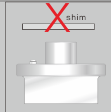
No shim after grinding
